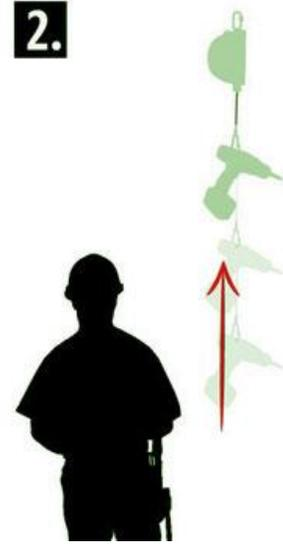
BY RELEASING THE USED APPLICATION, IT WILL TURN BACK TO ITS INITIAL POSITION.
